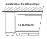
Cut out the upper part of the pump to fit the installation space. In the event the length needs to the air conditioning unit using a cutter. be extended, connect the duct afterwards
