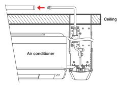
Run the insulated refrigerant pipes through the knock out tabs and up the inside of the trunking. use cable ties as required to secure the pipe.
